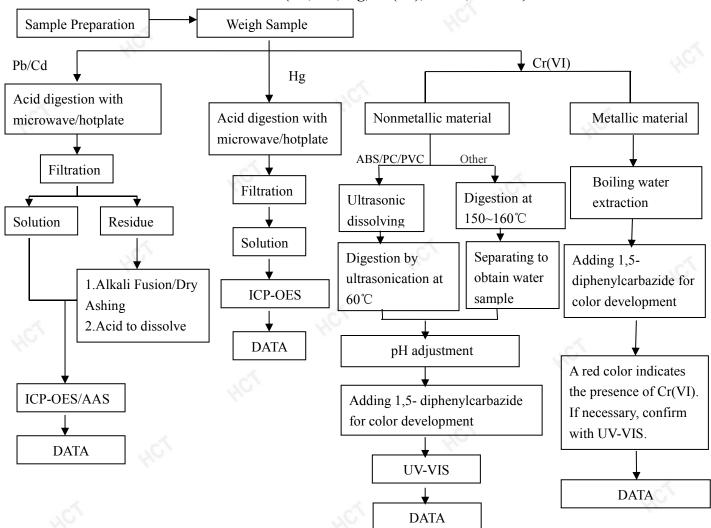
These sample were dissolved totally by pre-conditioning method according to above flow chart(Cr(VI) test method excluded)
