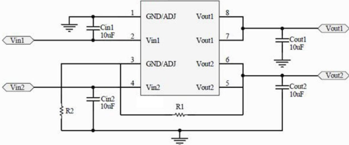
BRCO1118SE has both fixed voltage version (1.2V, 1.8V, 2.5V, 3.3V, 5V ) and adjustable voltage version. The input and output capacitors of each channel can be either tantalum, electrolytic or ceramic capacitor.
